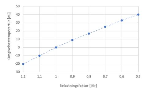
Assuming, for example, an average temperature during a summer month of 20°C, the maximum load factor of the transformer must be around 0.75.
